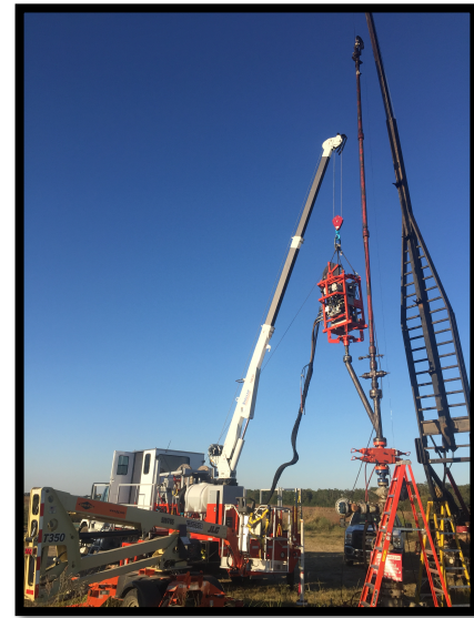
Figure 1-- Figure 1-- Y-Body Rig Up with Injector and Wireline
